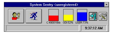
The leftmost button is used to logon and logoff. The next button is used to launch DOS or Windows programs. After the resource graphs is the Exit button followed by the Setup button.
